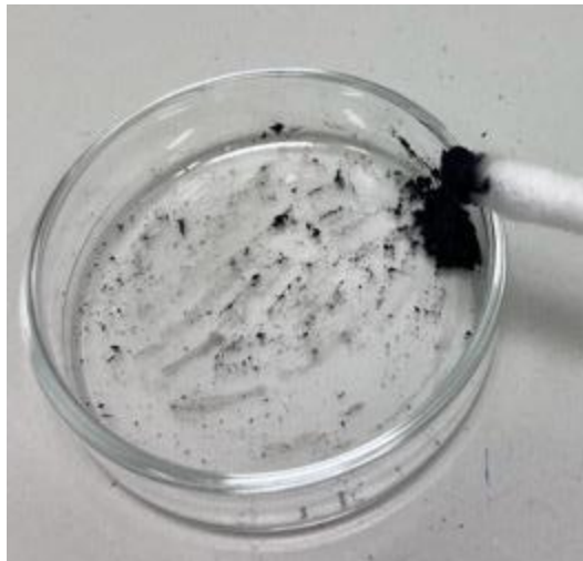
Straw ash mixed with deionised water as a polishing paste.
